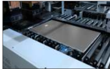
Longer grippers Automatic side leaning positioning, intelligent avoidance of drilling position, material grabbing speed up to 140m/min, really improving efficiency.
