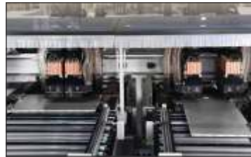
Double workstation Max processing width 1220mm/800mm min.space 64mm when two upper drill packages working .
