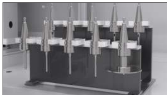
ATC double-layer 10-post ATC, meeting the fast tool changing needs of various machining processes;
