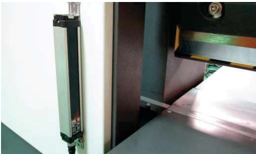
SAFETY LIGHT BARRIER OF KNIFE AND PACK BEAM IN FRONT
