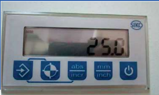
MAGNETIC SCALE FOR ACCURATE LINEAR POSITION MEASUREMENT OF THE FENCE
