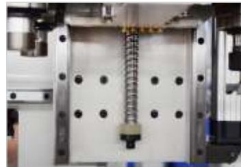
Motion mechanism Transmission mechanism: z-axis adopts ball screw, with high movement precision and compact structure.
