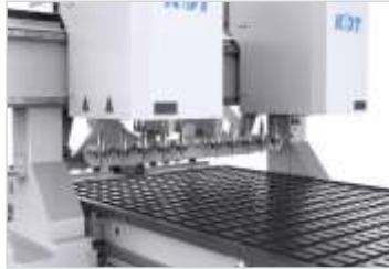
Tool library configuration Each spindle is equipped with 6 knives, reasonable distribution, non-interference.
